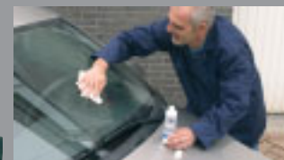
After cleaning the glass thoroughly finish the pre-treatment with the Aquacontrol Pre-Cleaner
